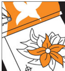
Rubylith - the analog way to mask a pattern.
